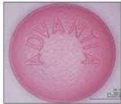
Surface Roughness Value, S_q = 5.41 A. Tablet Coated with Advantia® Preferred HS Coating
