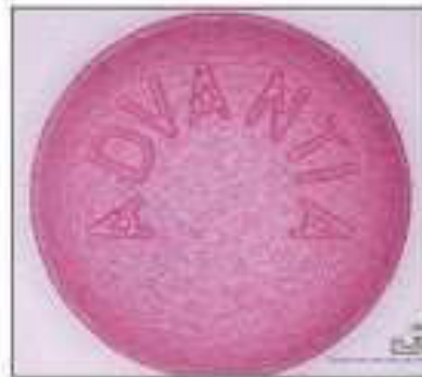
Surface Roughness Value, S_q = 8.40\mu m B. Tablet Coated with Polyvinyl Alcohol (PVA)-based Coating
